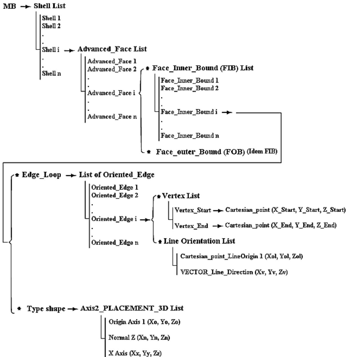
**Figure 3:** Translation of CAD data files into object-oriented data structure
