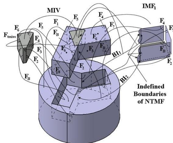
Figure 6: Analysis of a component obtained from the interaction between two Blind-pockets
