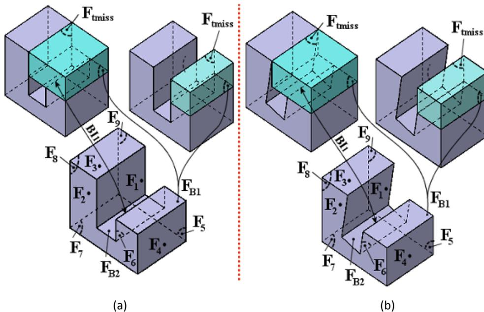
**Figure 7:** limit location of the Face Missed  $F_{miss}$  by the interaction between two MF: slot and step determined and a suitable virtual Face  $F_V$  that substitutes  $F_{miss}$  can be therefore stored.
