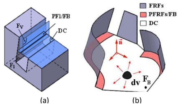
**Figure 8:** Model for rebuilding interacting features: a) virtual Face that materialize the possible position of  $F_{miss}$ , b) Domain of construction by taking Account the faces boundaries surrounding the  $IMF$
