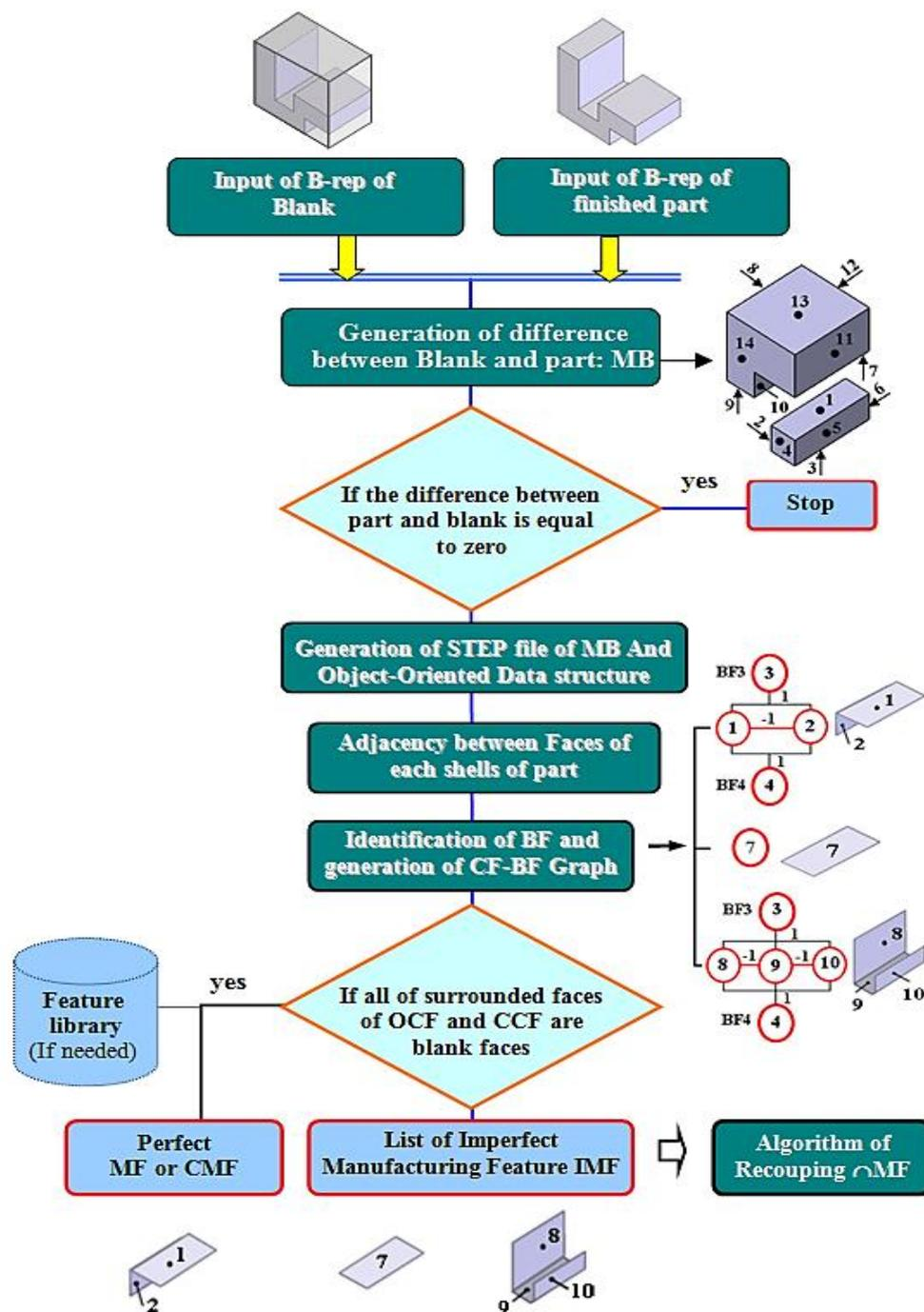
Figure 10: Algorithm 1: Flowchart for extraction of perfect MF and CMF
