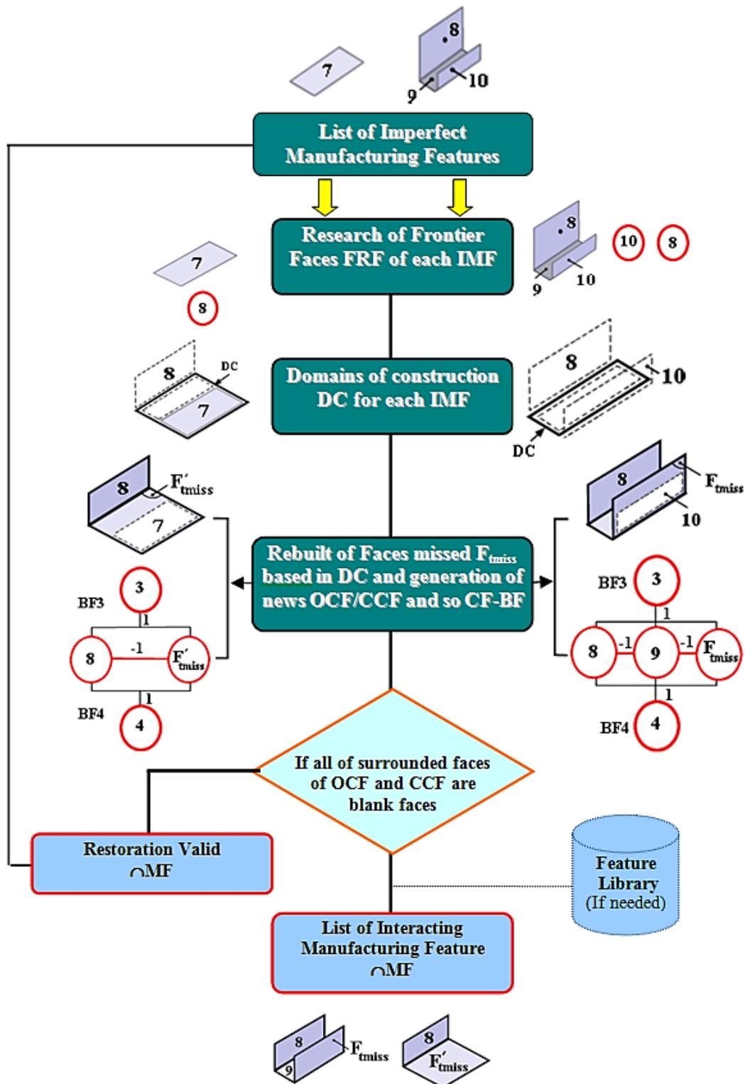
Figure 11: Algorithm 2: Recouping of the Interacting Manufacturing Features  $\cap$ MF
