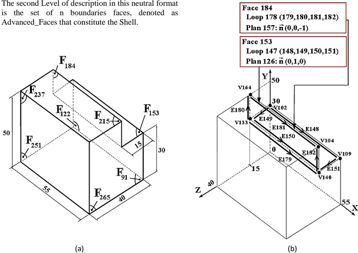
Figure 2: A sample part for explanation of STEP format
