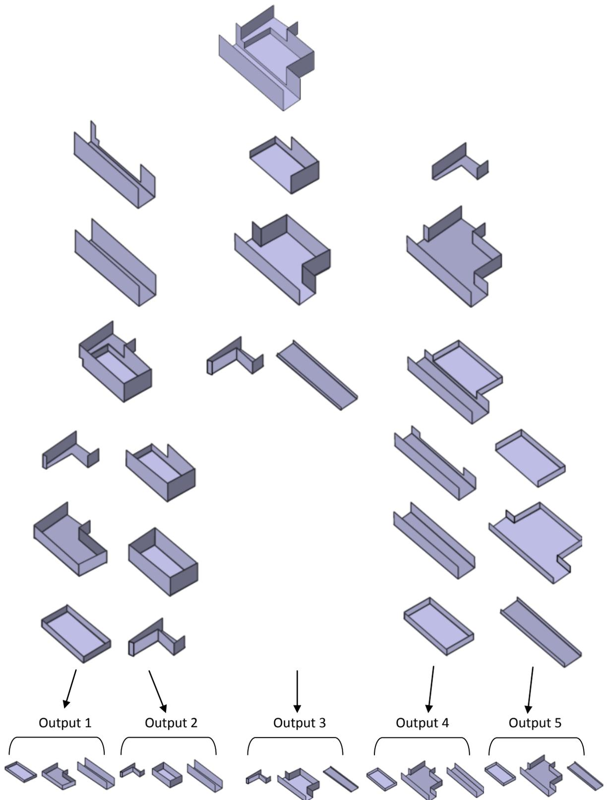
**Figure 13:** Manufacturing Feature derived from application of Algorithm
