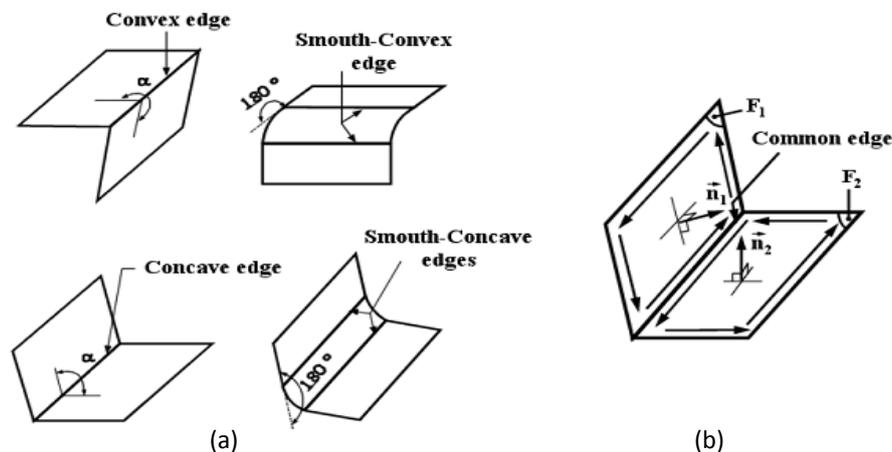
**Figure 9:** Edge classification (a) and concavity test of shared edge between two adjacent faces  $F_1$  and  $F_2$  based on right hand rule (b).
